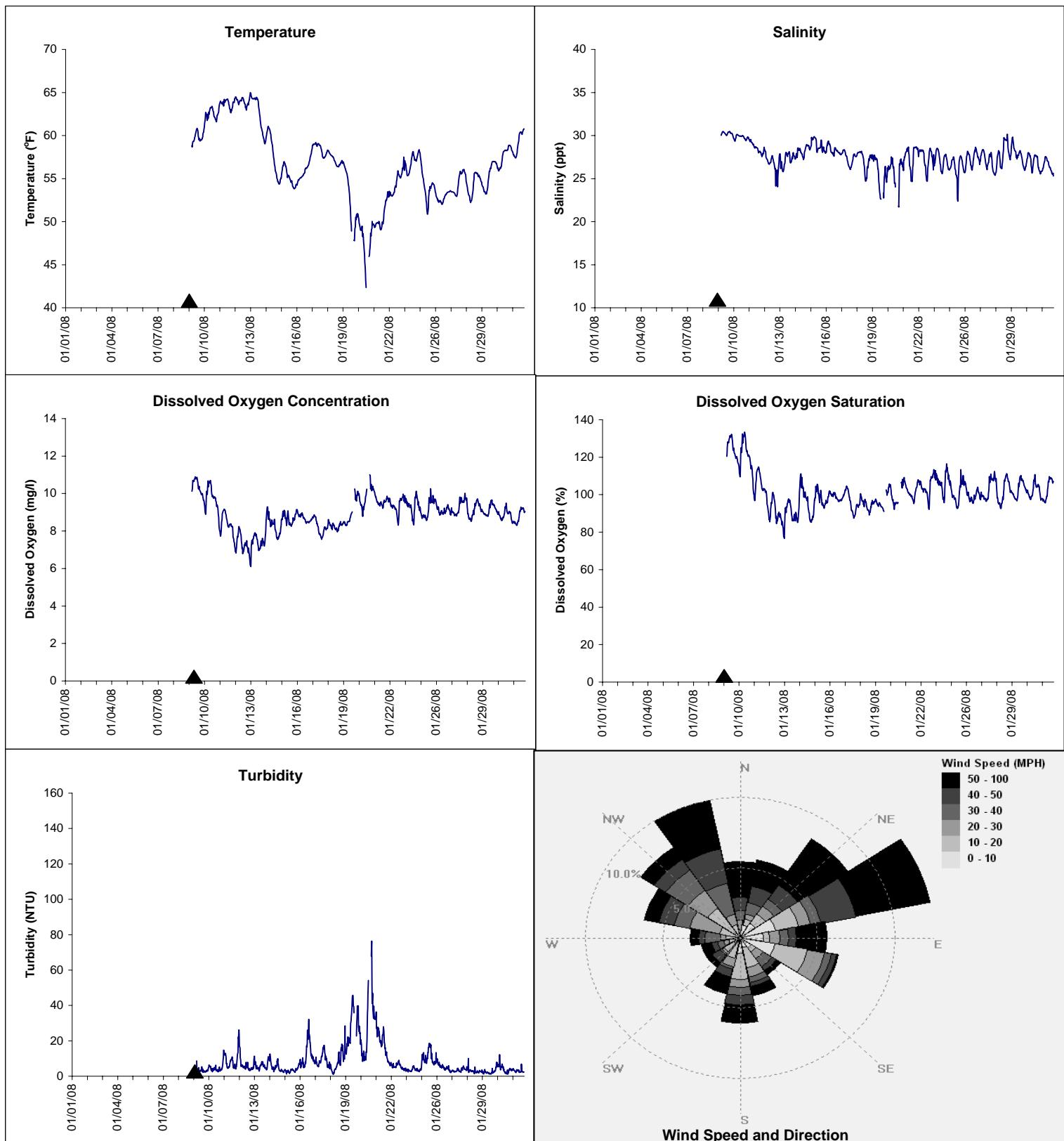
▲ Monitoring Equipment Exchanged (sonde deployment)
