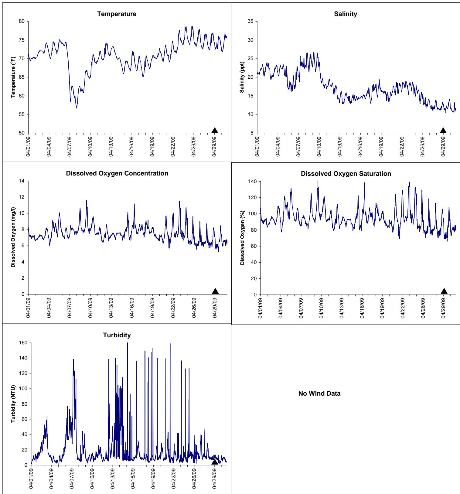
▲ Monitoring Equipment Exchanged (sonde deployment)
