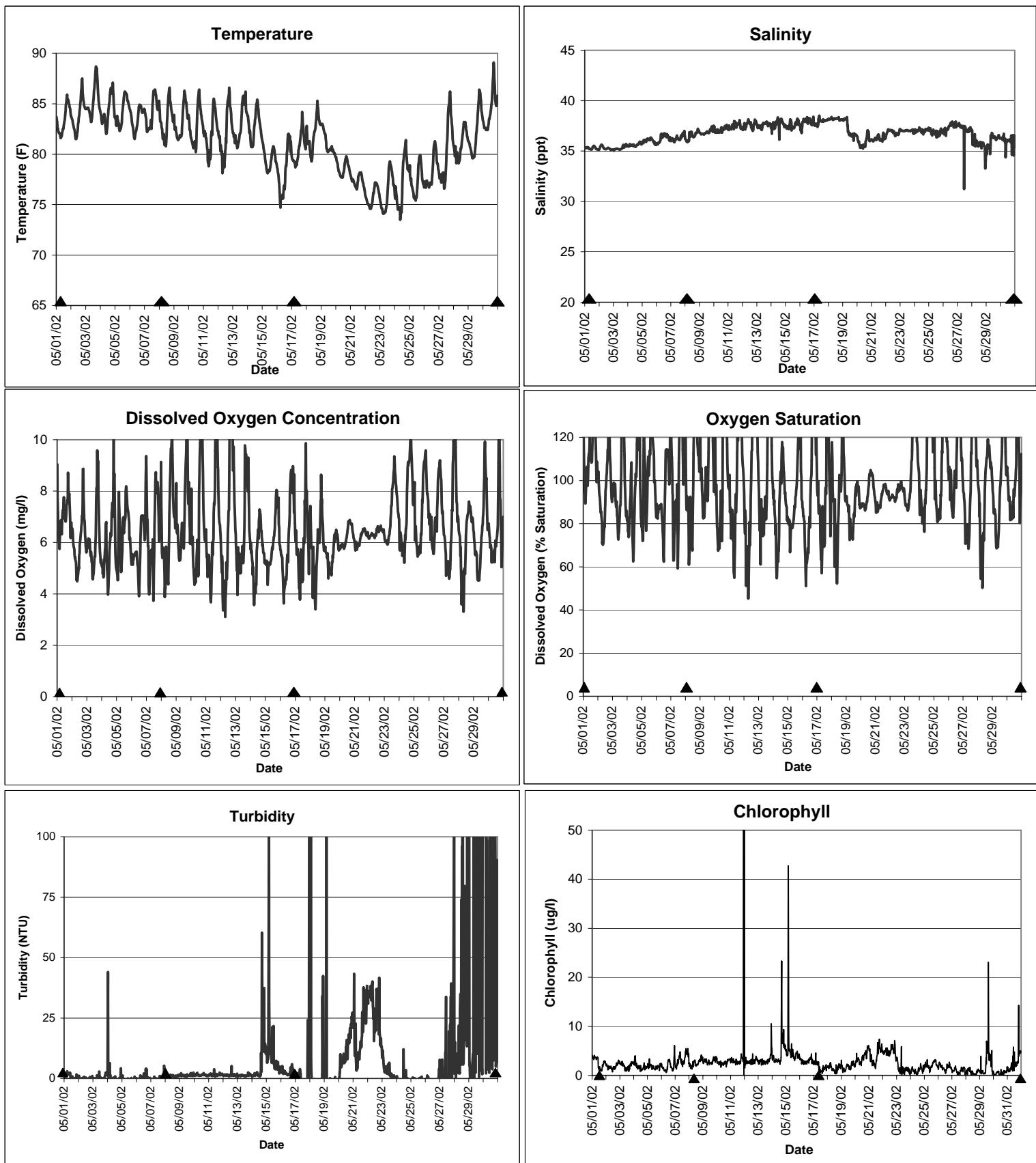
▲ Monitoring equipment exchanged (sonde deployment)
