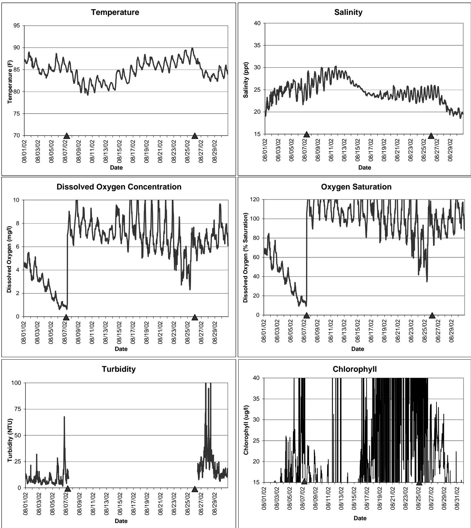
▲ Monitoring equipment exchanged (sonde deployment)
