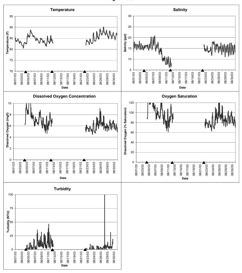
▲ Monitoring equipment exchanged (sonde deployment) Refer to the QA/QC log for additional information.
