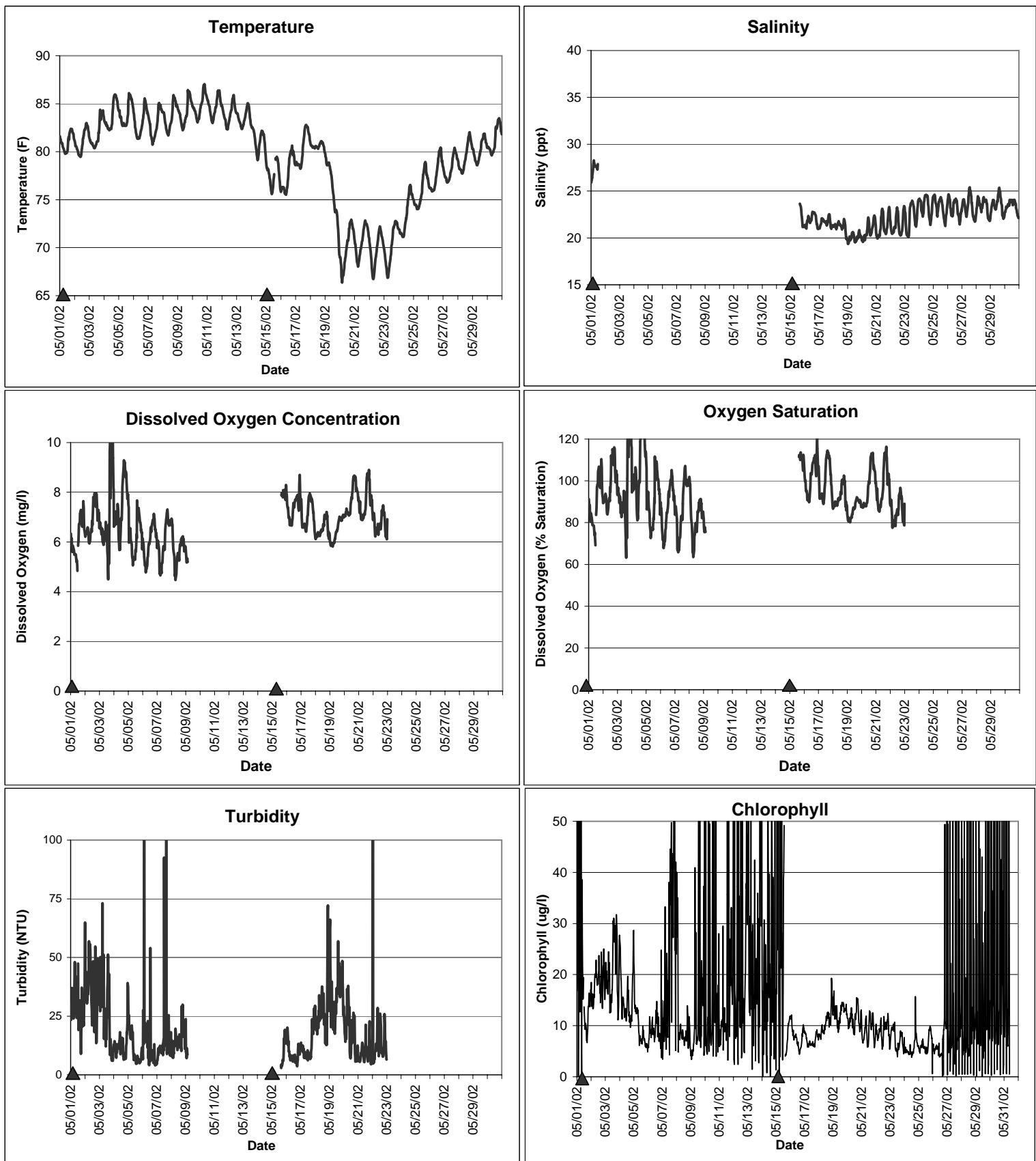
▲ Monitoring equipment exchanged (sonde deployment)
