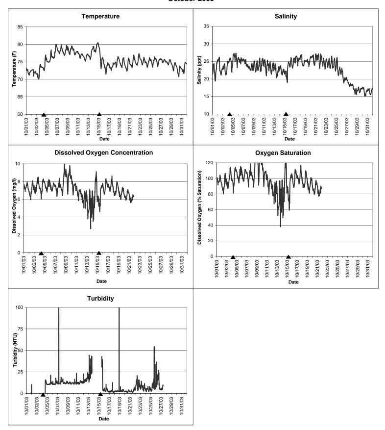
▲ Monitoring equipment exchanged (sonde deployment)
